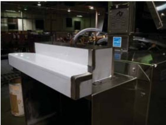
Vent attachments to end shield, 4” x 16” opening
