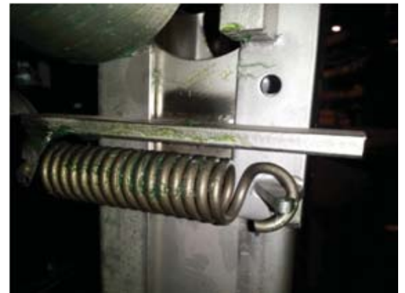
Rocker arm slip clutch spring, hook to bar weldment
