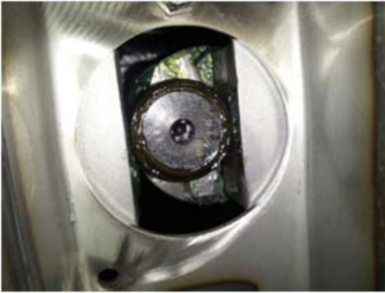
Cam bearing screws into cam block B
