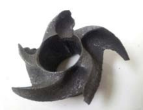
Impeller damaged from high acid solution
