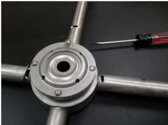
Remove 4 screws and lift top shell
