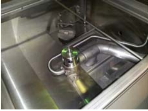
Showing spray arm base & transfer tube
