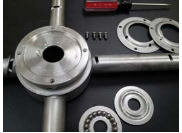
Races are interchangeable, capture shells are also
