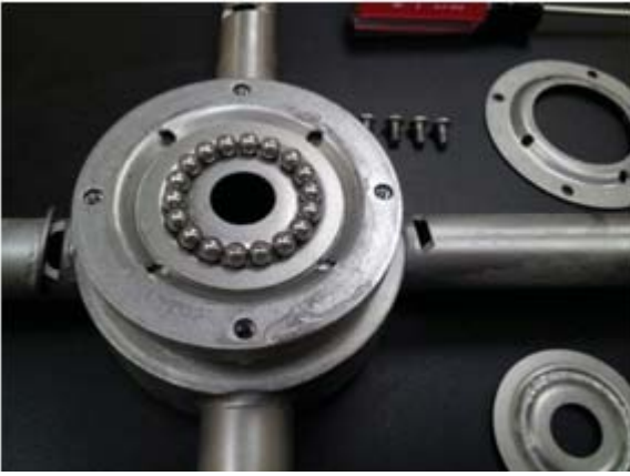
Top race removed, ball bearings for replacement
