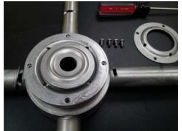
Remove top shell, exposing top bearing race
