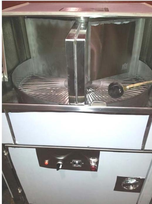
The red “START” button on the front of the lower access door will start the cycle. Watch the temperature indicator located behind the lower inspection door on the tank wall, the minimum required is 120F at the machine. If the temperature does not meet minimum, check the building water heater.
