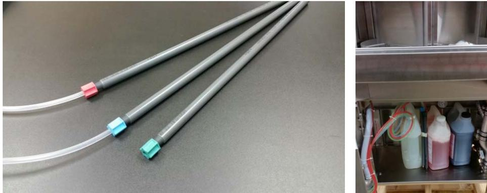
Check the level of the chemical containers, make sure the lines are put in the proper color coded chemical container and secured to the container, RED for detergent, BLUE for rinse aid, GREEN for sanitizer
