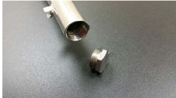
Make sure all the spray tips are open by using a tooth pick to push any clog into the center of the arm, after rinsing out the arm, screw the end caps into both ends of the spray arm.
