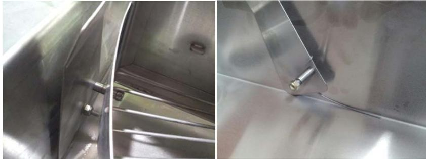
**MANUALLY TURN**— the carousel until the loaded glasses are in the washing compartment . Proper alignment is indicated when the latch detent pushes into the notch of the carousel wheel.
