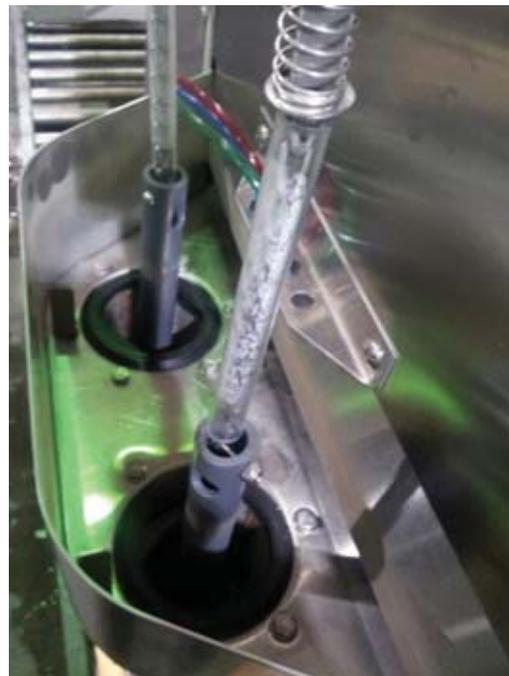
Dual drain balls, sumps, and pump filters
