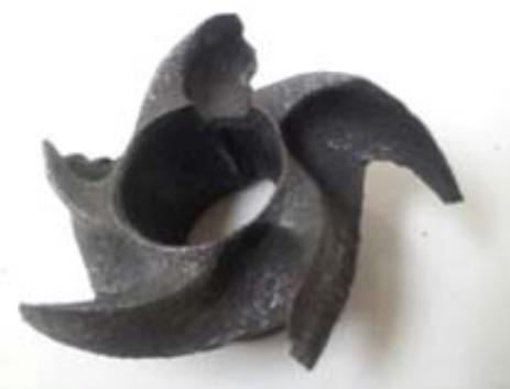
Impeller damaged from high acid solution
