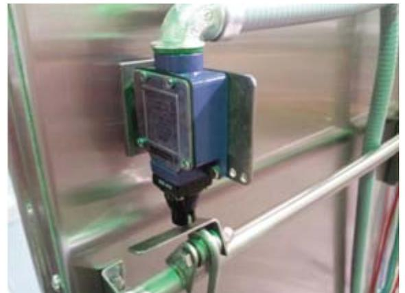
5-AGS Door cut-off switch and lever arm
