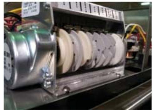
The left photo shows arrow is pointed at the left-side wheel of the cam which is used to lengthen or shorten the low cam or the time ON for the respective switch. Center photo shows high-cam & low-cam notch. Adjustable cams are colored either black or gray.
