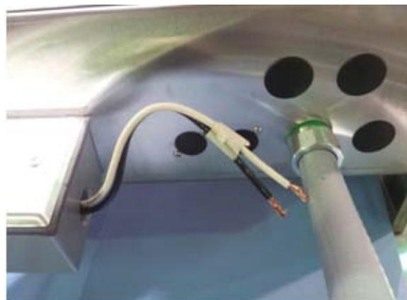
Showing power connection for 120v wiring
