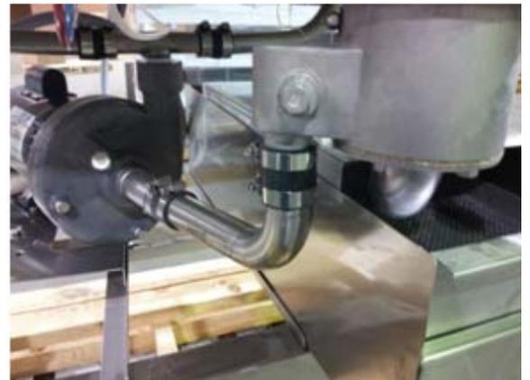
Single Pump, intake and discharge manifolds
