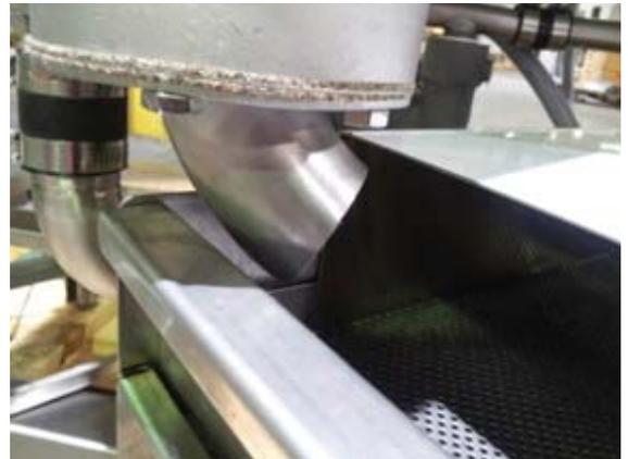
Correct alignment for sump to box
