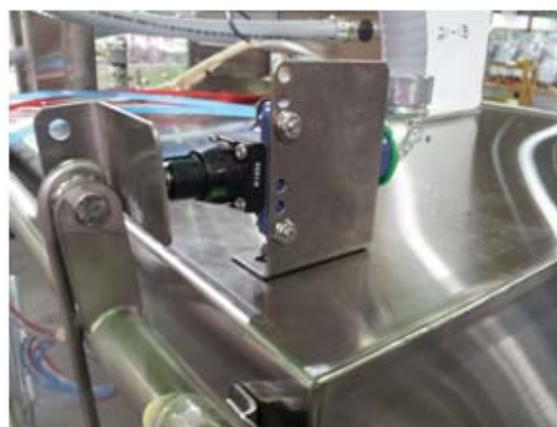
5-CD Door cut-off switch and lever arm
