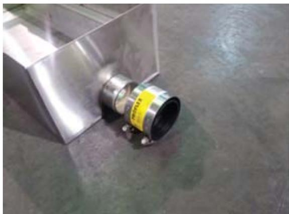
Showing the scrap box rear exit drain hub connection
