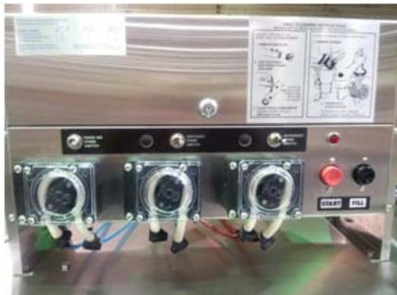
Showing the control box with chemical pumps, prime switches, red start and black fill switch
