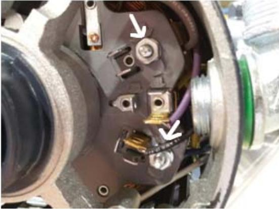
Showing connection points in 1 HP, 120v motor
