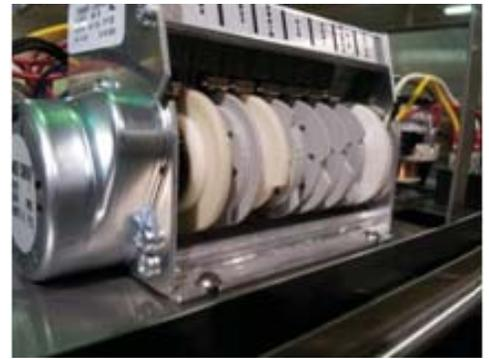
The left photo shows arrow is pointed at the left-side wheel of the cam which is used to lengthen or shorten the low cam or the time ON for the respective switch. Center photo shows high-cam & low-cam notch. Adjustable cams are colored either black or gray.
