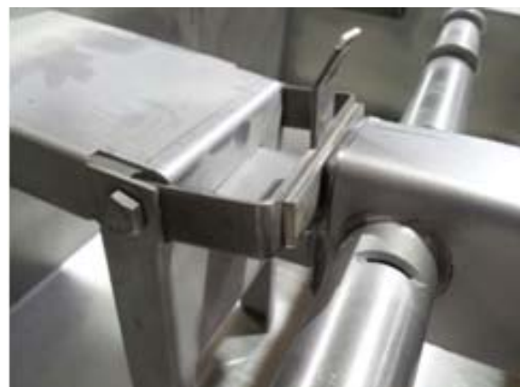
Arm resting in “T” index with latch down
