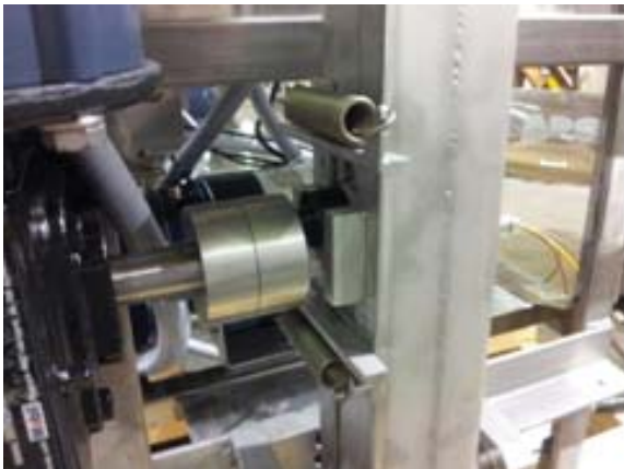
Conveyor drive, cam blocks, bearing, clutch springs (use caution)
