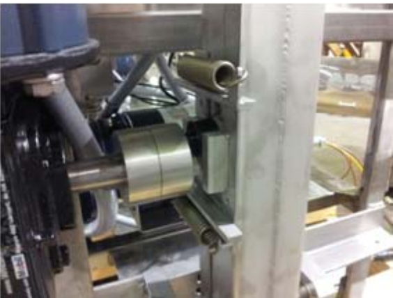
Conveyor cam blocks A & B
