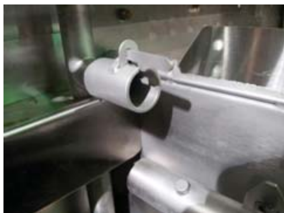
Showing pumped rinse manifold locking tab
