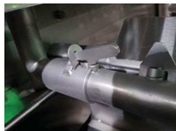
Rinse arm index notch, latch will drop as arm is pushed in
