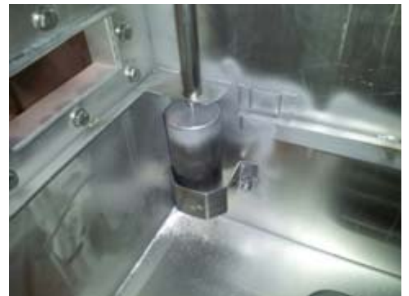
Wash tank float and tank overflow
