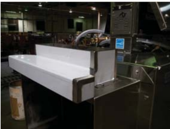
Vent attachments to end shield, 4” x 16” opening
