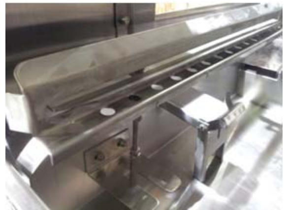
Wash tank sequence bar, pendulum with magnet
