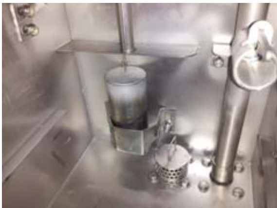
Rinse tank float, pump filter, pumped rinse manifold
