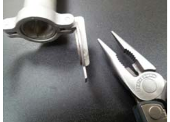
Straighten tab in line with the coin edge to tighten
