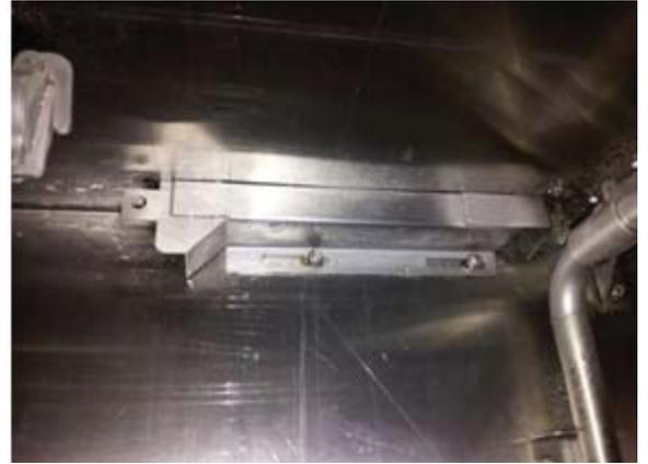
Showing “float” switch that controls fill water & heater
