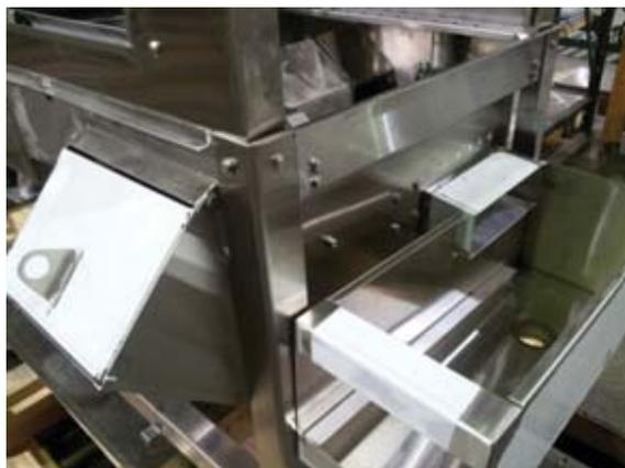
ADC-66 power scrapper, overflow to scrap box
