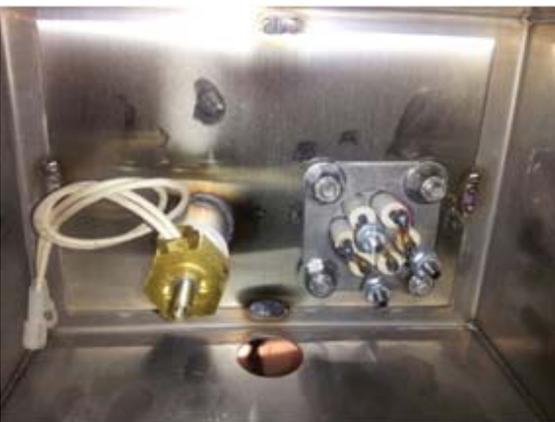
Wash tank thermostat, rotate center rod Left to increase
