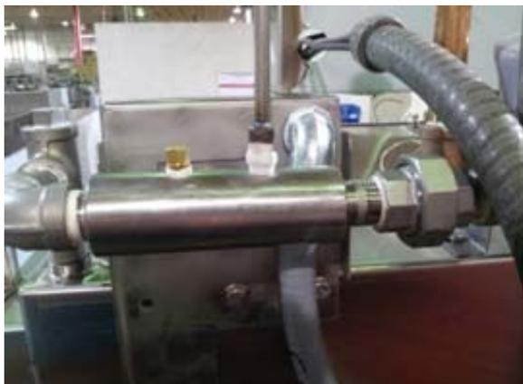
Mixing chamber with two 1/8" pipe threaded ports
