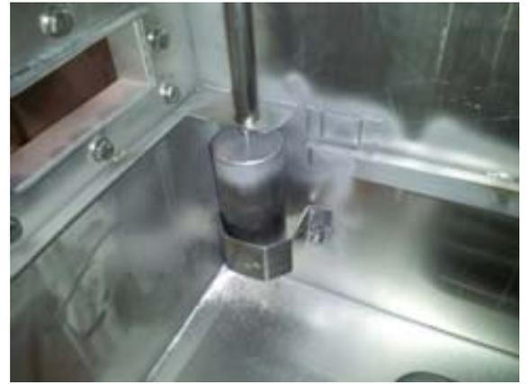
Wash tank float and tank overflow
