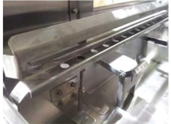
Wash tank sequence bar, pendulum with magnet
