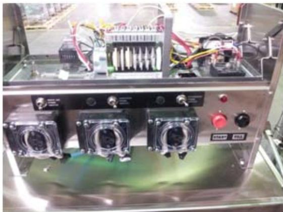
Showing control box, chemical pumps, prime switches
