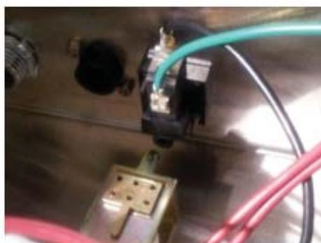
Optional Chemical Alarm switch, buzzer
