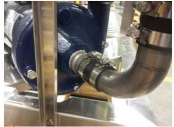
Pump intake and connector sleeves with clamps
