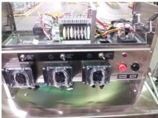
Showing control box, chemical pumps, prime switches
