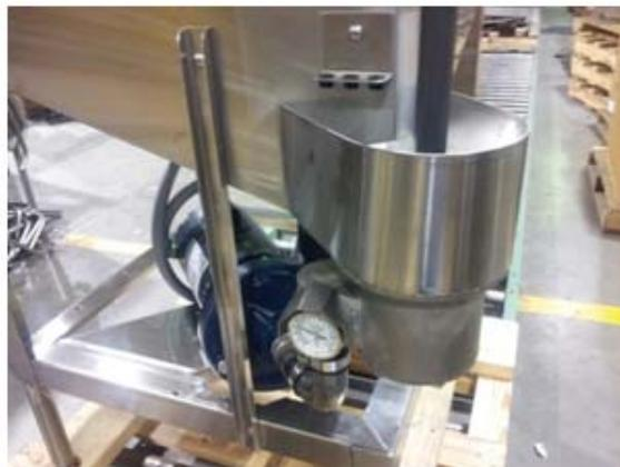
Showing AF-ES sump, drain ball, thermometer
