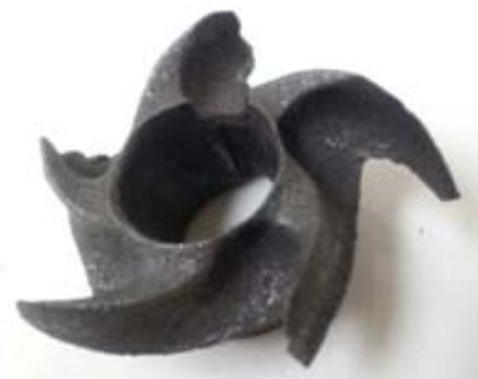
Impeller damaged from high acid solution
