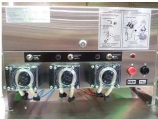
Showing the control box with chemical pumps, prime switches, red start and black fill switch, chemical tubes
