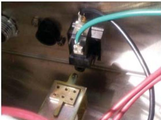
OPTIONAL Chemical Alarm switch, buzzer
