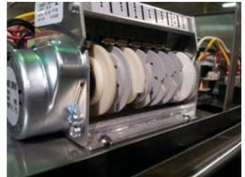
The arrow is pointed at the left-side wheel of the cam which is used to lengthen or shorten the low cam or the time ON for the respective switch. Adjustable cams are colored either black or gray.
