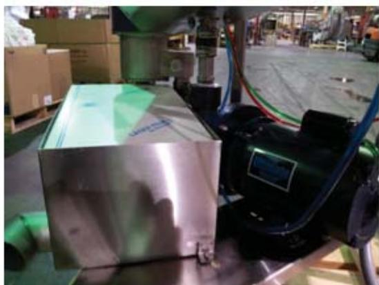
Rear view of installed side exit ES scrap box
