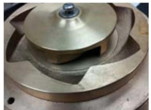
Diffuser removed, centrifugal Impeller
