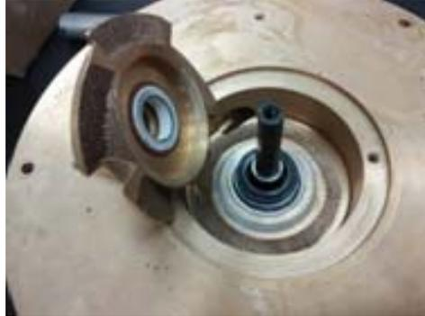
Ceramic seal pressed into propeller
