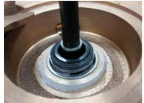
Graphite seal pressed into pump base
