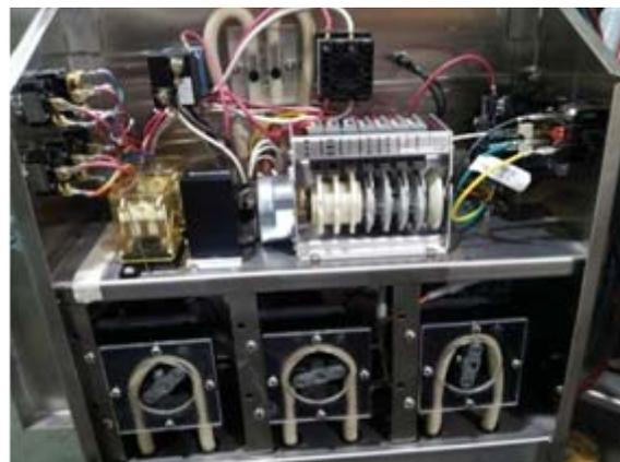
ASQ control box with cover removed
