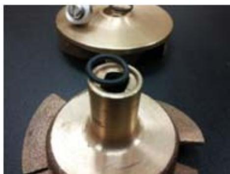
Small o-ring on top of propeller
