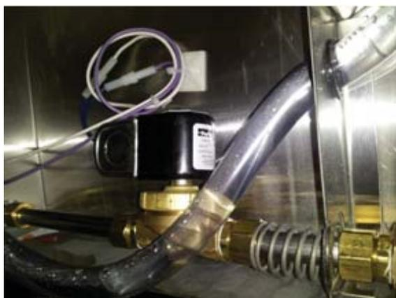
Showing ½" H<sub>2</sub>O solenoid, also plastic drain tube
