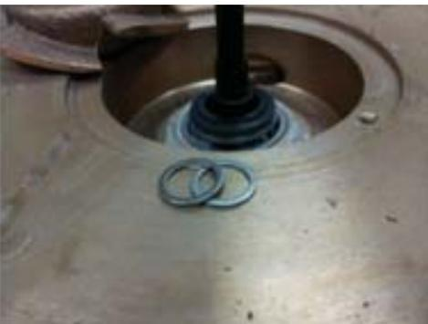
2 Spacer washers under propeller
