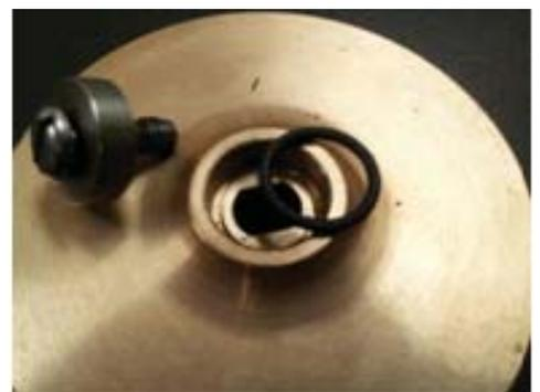
Large o-ring in top of impeller
