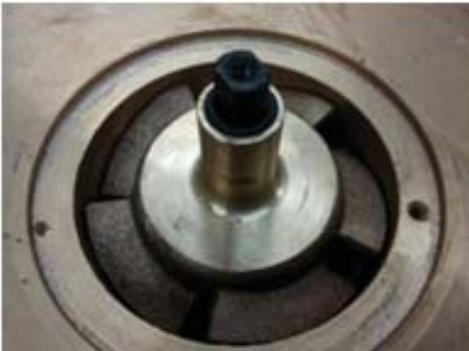
Drain axial propeller, o-ring on shaft
