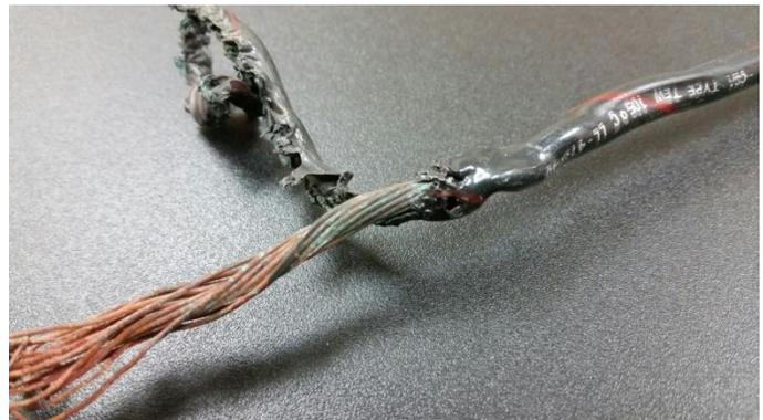
These are burned wires and should not be reused to transfer electrical power to motors or heaters.
