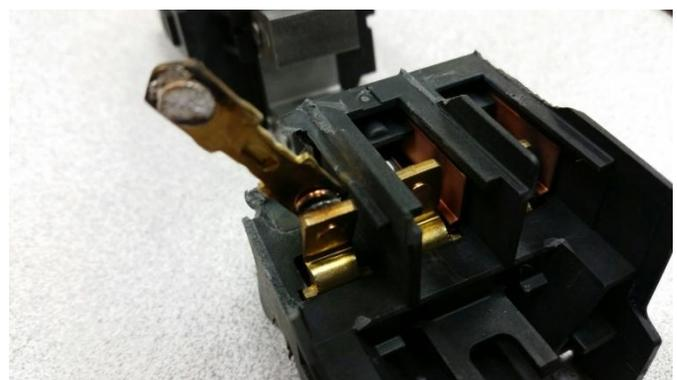
Showing inside of the contactor where contact points burned together (welded). This was caused by loose screw terminal.
