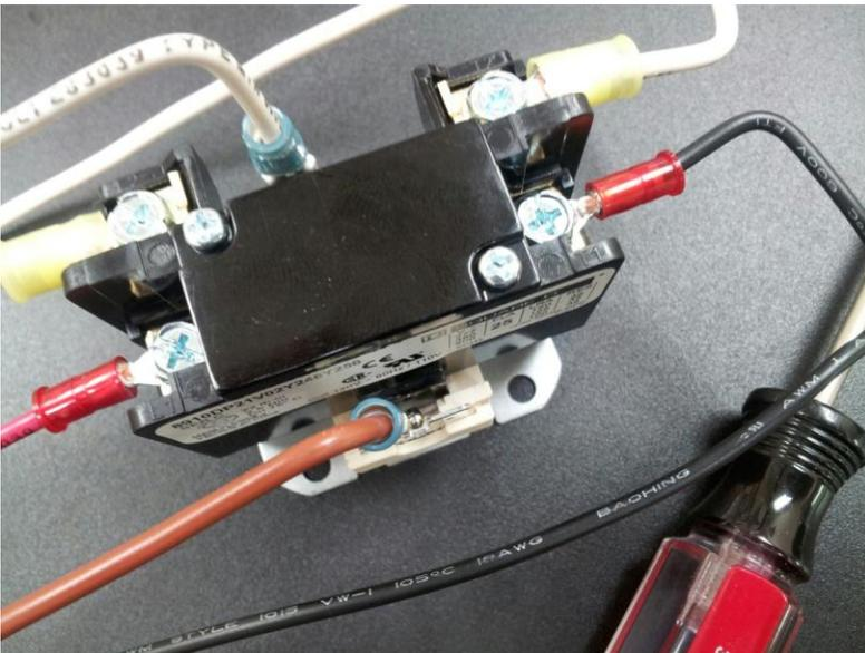
Showing correct wiring of contactor, NOTE white neutral wires connect across the common bar and red power wire connects across contact points (points are under black cover) to black wire for the motor. Often, by mistake these wires are reversed in positions when a replacement contactor is installed, causing the motor to run any time power is turned on.
