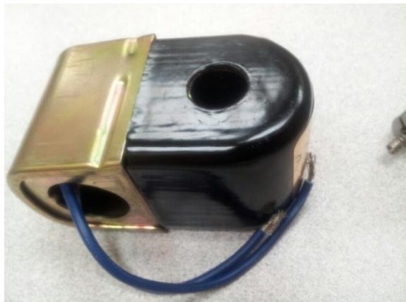
If voltage is at the coil but plunger will not lift, bad coil
