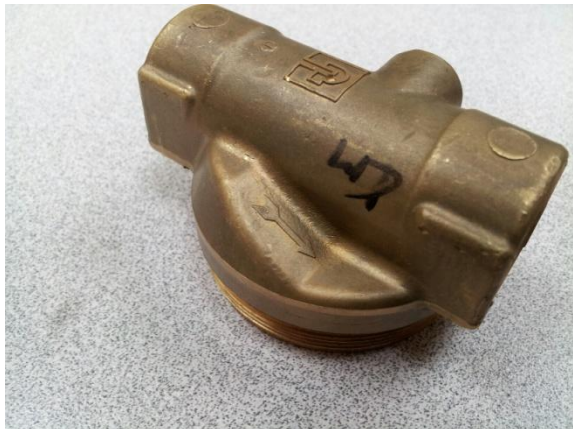
Installing valve wrong way, see arrow flow direction
