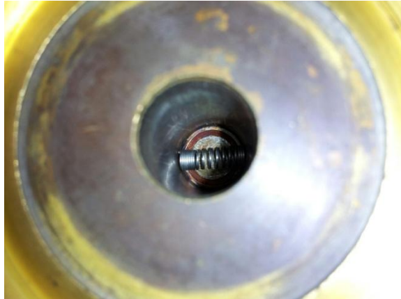
Failing to remove spring lodged in tube
