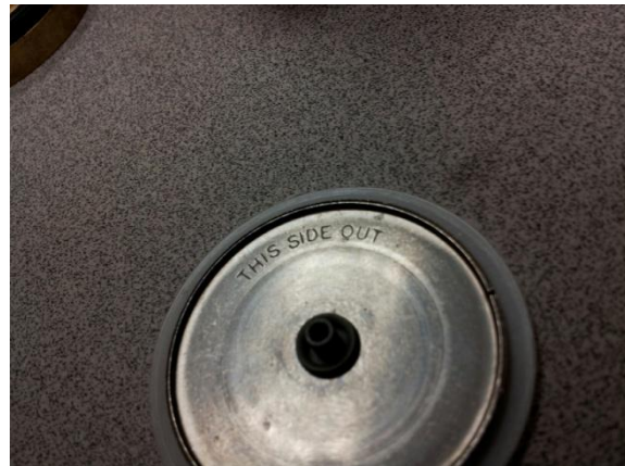
Installing diaphragm upside down, see lettering up
