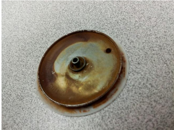
Errors are returning a corroded diaphragm to service.
