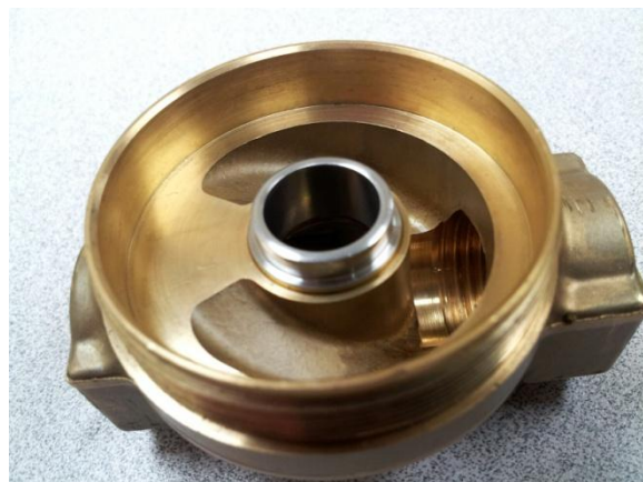
Remove any material or debris from the body. Inspect
