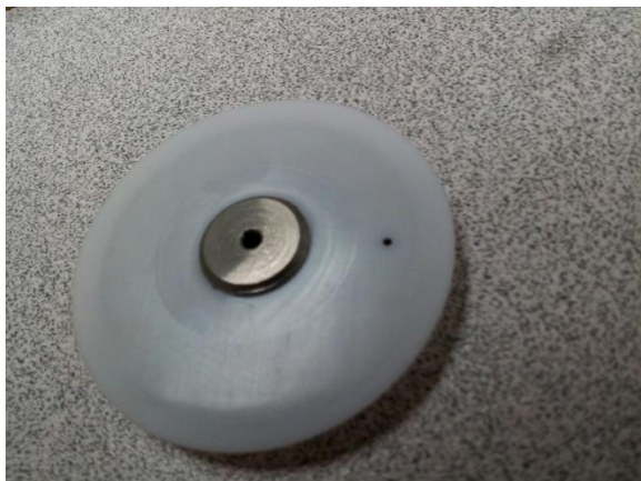
Turn over the diaphragm inspect near the rivet head
