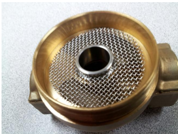
Remove the o-ring retainer, remove the screen the center ring for cuts or damage to the surface. If the stainless seat (center ring ) is rough or cut, the valve body must be replaced.
