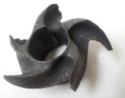
Impeller damaged from high acid solution
