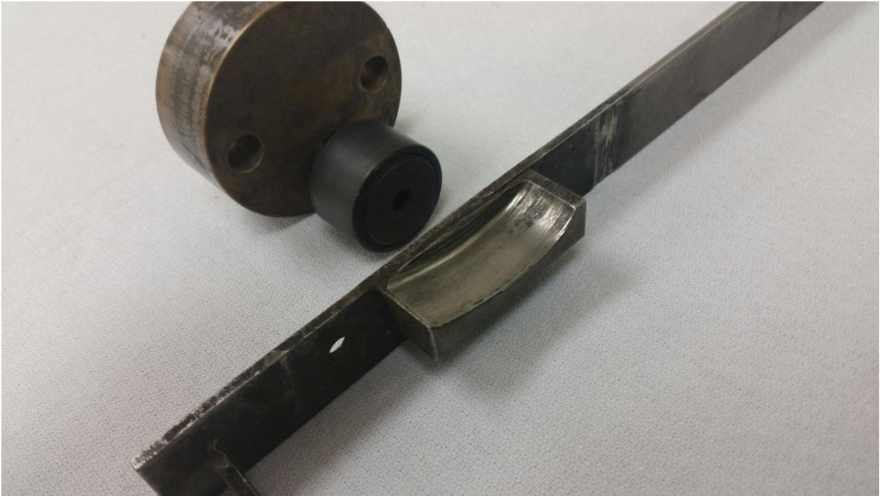
Cam block B (281-6135), Cam Follower Bearing (281-6201), Slip Clutch Bar (285-6134) showing half-moon groove cut by rusted brg.
