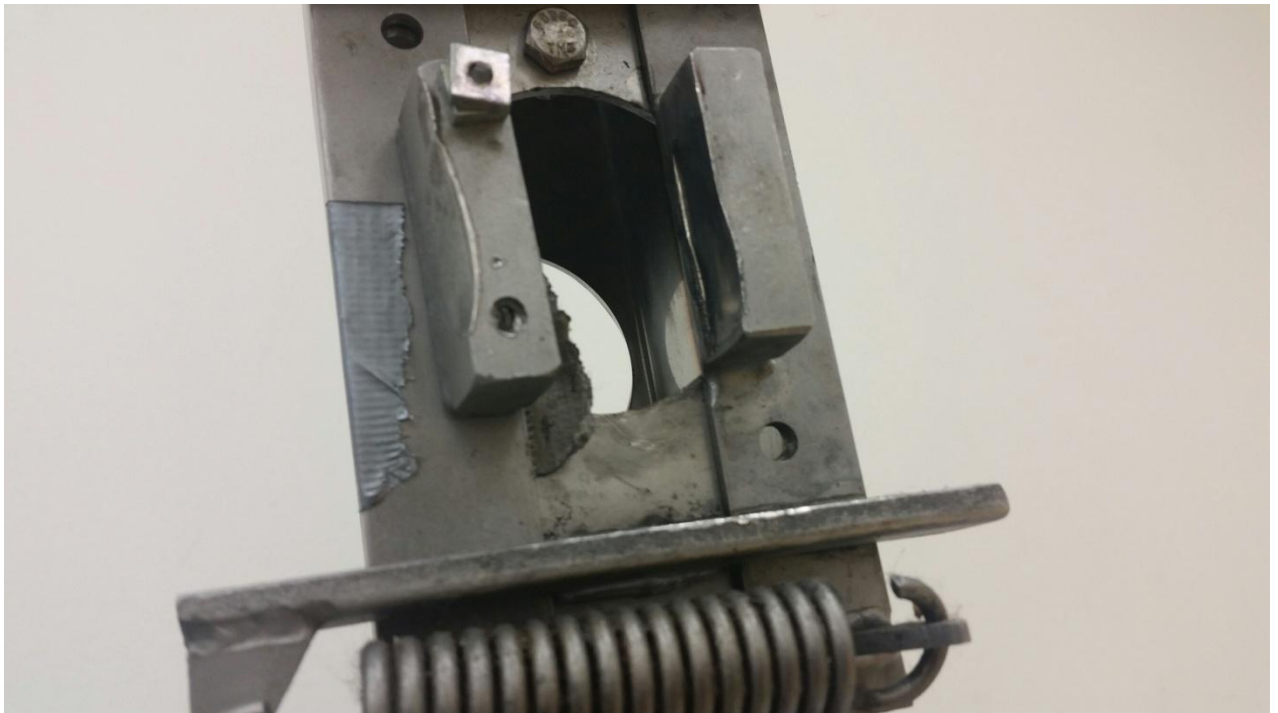
Rocker arm (285-6133), worn Slip Clutch Bars (285-6134) showing attempted repair using screws and duct tap Lower Slip Clutch Spring (298-3001)
