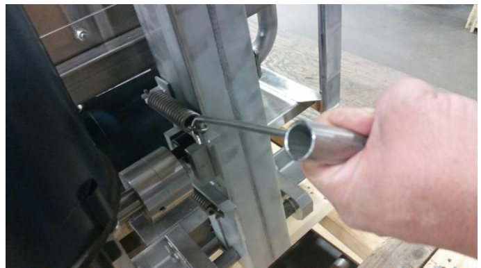
Tool will hook around spring end to pull over the retainer ear
