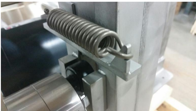
Conveyor upper slip clutch spring (298-3001) w/ 30 ft/lbs pull
