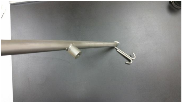
Double hook end under frame member
