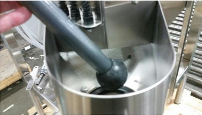
**First:** empty the water from the sump by lifting the drain ball. Place the drain ball back in the sump when the water is gone.
