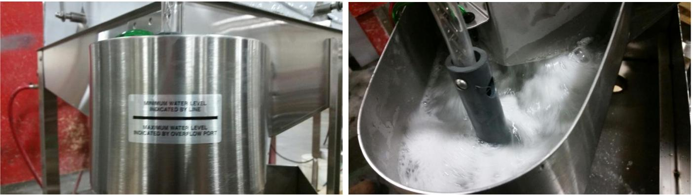
**Third:** The water level decal indicates the approx fill level. Release the fill button when this level is reached. Record the seconds it took to reach the fill level.
