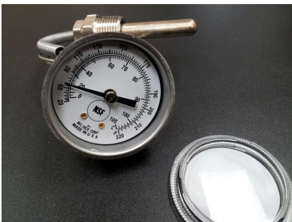
Remove lens cover to calibrate if needed
