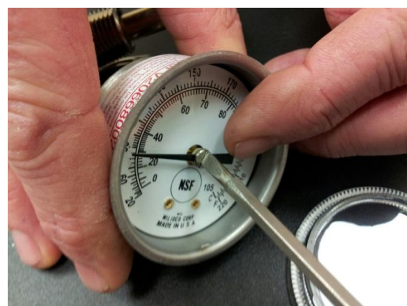
Hold center rod stationary while turning pointer
