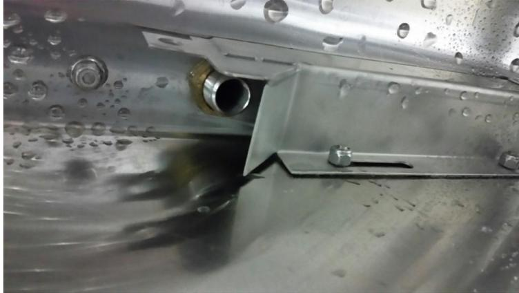
Please note in picture #1 looking up, the adjustment studs are shown at the far left of the slots (meaning the diverter inlet duct (285-6147l-r, 285-6127r-l) is moved to the far right of this machine--a L-R conveyor) and the water pipe exit is fully open to drop into the wash tank. Adjusted as shown means the rinse tank would receive no water and the machine would continually fill, not shutting off.
