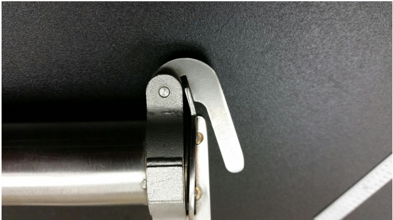
This picture shows a loose endcap that won't stay closed because the tab is bent in toward the tube.
