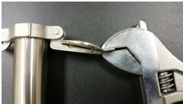
Bend the tab of the endcap straight again
