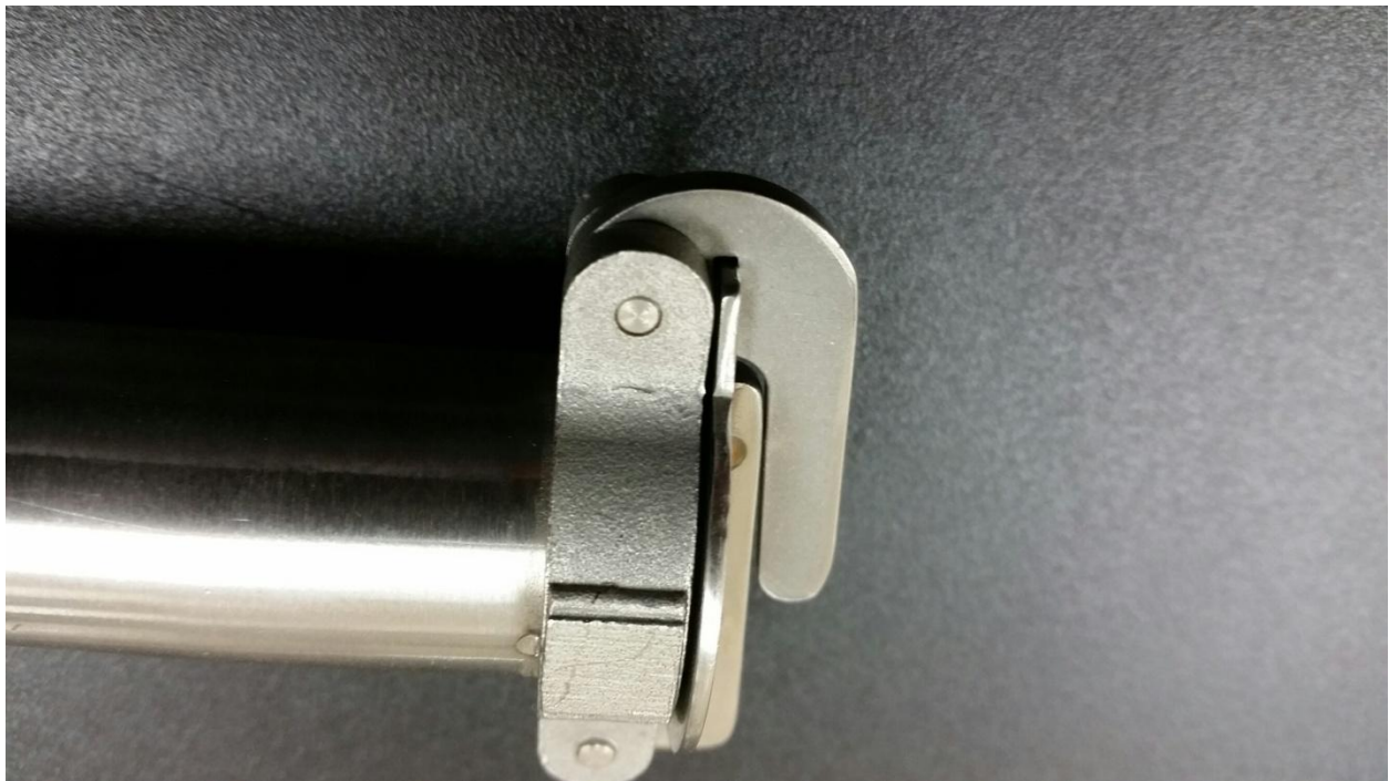
Showing a tight snap-action captive endcap in the closed position. When the endcap is closed properly, it is normal for some water to spray out from around the cap; this will act as the last spray jet on the arm.
