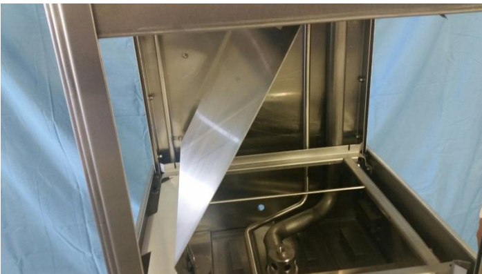
Tray track may need to be lowered to fit shield inside
