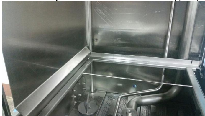
The shield becomes the tray track rail for the racks
