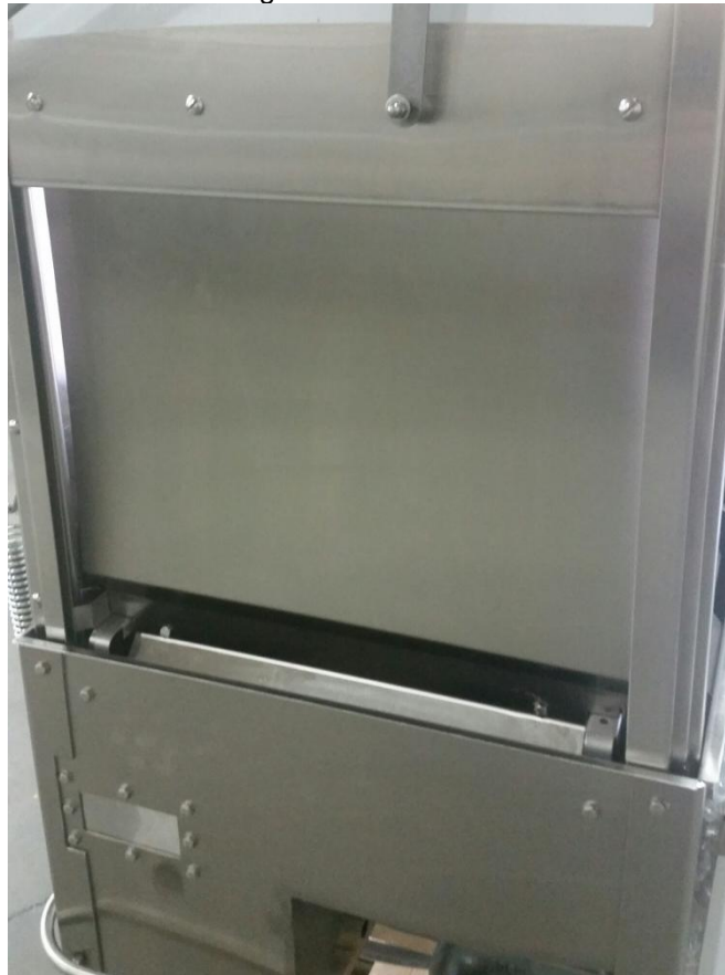
Showing finished install of shield
