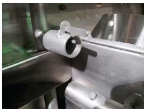
Showing pumped rinse manifold locking tab
