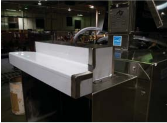
Vent attachments to end shield, 4" x 16" opening
