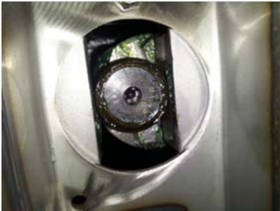
Cam bearing screws into cam block B
