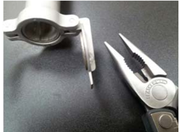
Straighten tab in line with the coin edge to tighten latch
