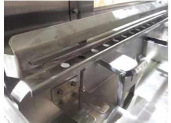
Wash tank sequence bar, pendulum with magnet
