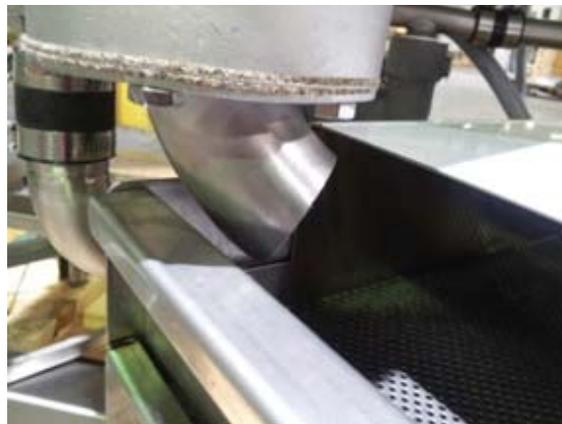
Correct alignment for sump to box
