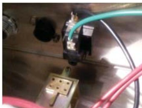
Optional Chemical Alarm switch, buzzer
