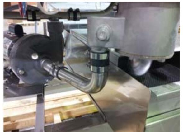
Single Pump, intake and discharge manifolds
