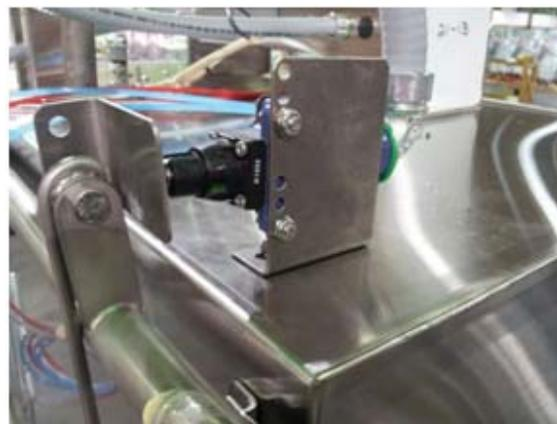
5-CD Door cut-off switch and lever arm
