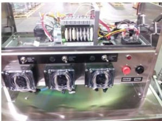
Showing control box, chemical pumps, prime switches
