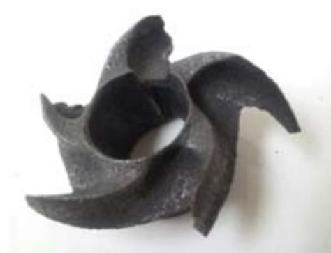
Impeller damaged from high acid solution
