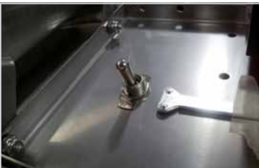
De-lime switch in control box
